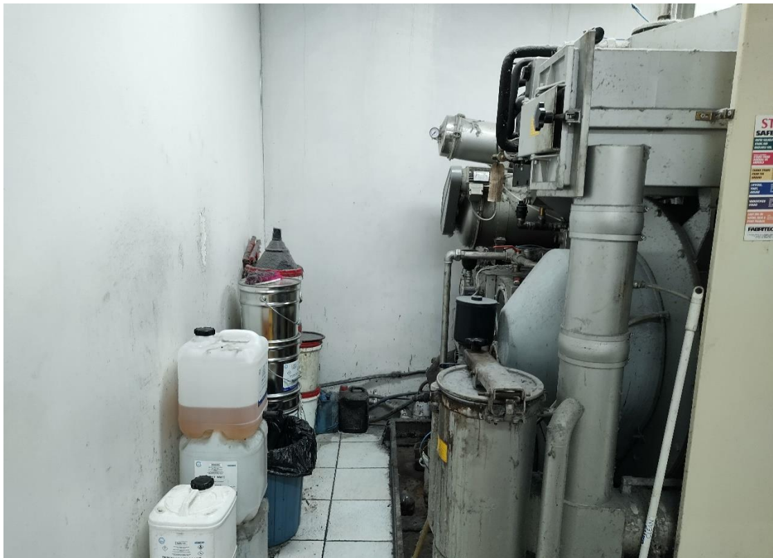
Photo 4: Interior of dry cleaner, storage of tetrachloroethene (PCE) containers
